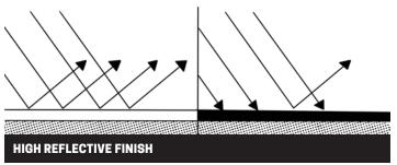
AlphaGrade's bright white finish can improve reflectivity up to 8x that of a gravel surfaced roofing system.
